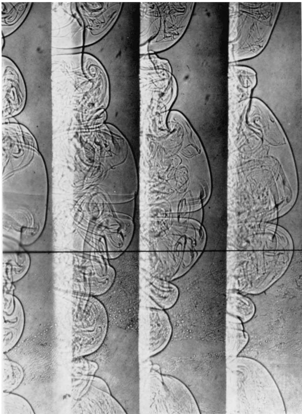
FIGURE 7. Part of a series of lobe shadowgraphs. \Delta\rho/\rho = \frac{1}{2}\% , H = 24 cm. Reproduced \frac{7}{8} full-size.
